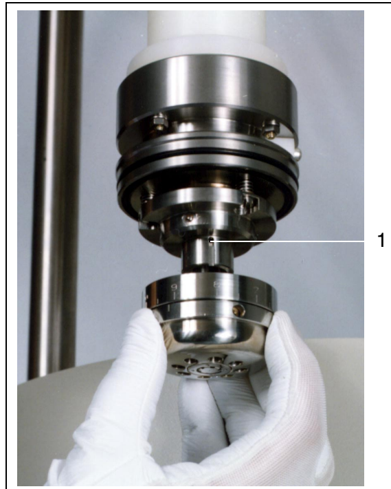
FIGURE 3-8 SECURING THE WEHNELT ASSEMBLY
