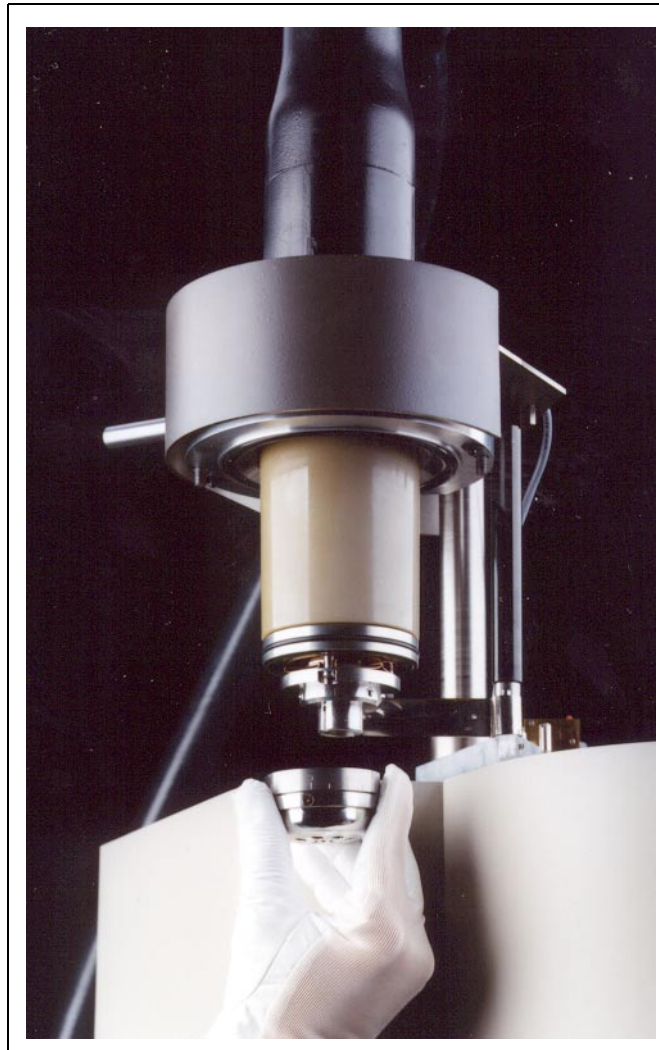
FIGURE 3-7 DISMOUNTING AND REMOUNTING THE WEHNELT ASSEMBLY
